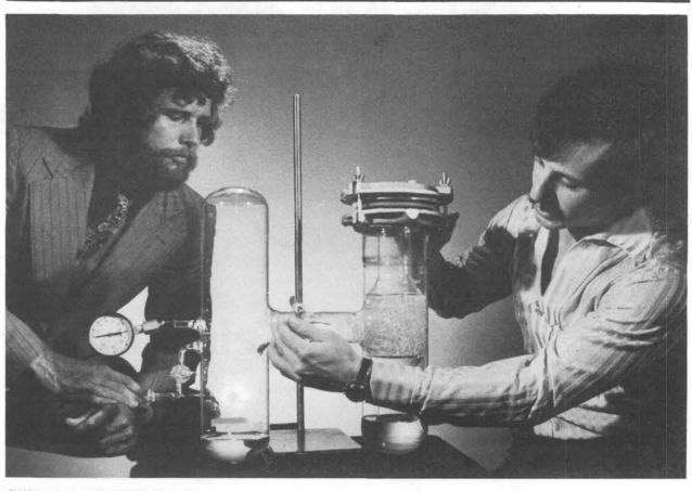
CHEMICAL HEAT PUMP holds the attention of Taz Bramlette (left, 8451) and Carl Hiller (8453). This working model contains sulfuric acid in right hand column, water in left. Allowing them to recombine produces heat.
